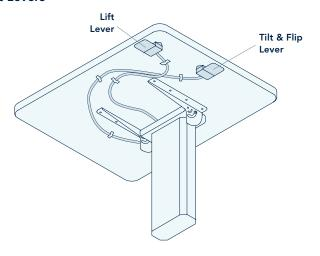
The Jimmy Table features **two adjustment levers**: The front lever controls lift and the side lever controls flip and tilt. Refer to **user guide** for instructions.
