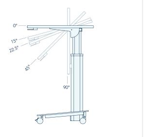
The Jimmy flip mechanism allows the tabletop to be **tilted and locked securely** at the following angles:  $15^{\circ}$ ,  $22.5^{\circ}$ ,  $45^{\circ}$  and  $90^{\circ}$ .
