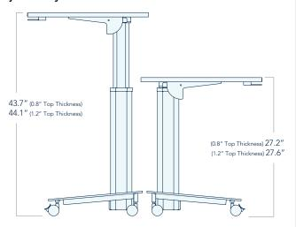
The Jimmy Table column features a constant force spring mechanism that includes a **safety break with integrated locking** that enables smooth and safe adjustment of tabletop height.
