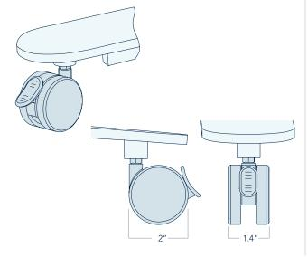
The Jimmy Table is equipped with with **four black 2" dia. casters**, including two locking casters in the front.
