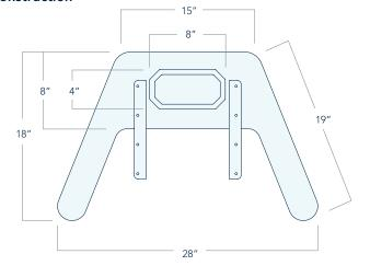
The Jimmy Table height adjustable base and column are made from formed steel and bolted together. The base can support a recommended **maximum** weight of 20 lbs. (in addition to the top.)
