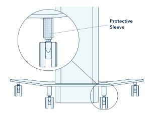
The Jimmy Table is equipped with **rubber sleeves** on the two back caster stems to protect the base when nested.
