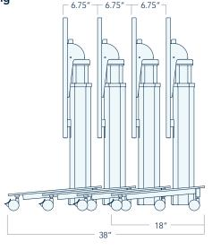
The Jimmy Table safely and easily flips down with the inclined base providing for **straight-on nesting**. Each additional nested table adds approximately 6.75" to the overall depth of all nested tables.
